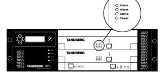
The system is ready for configuration once the Power and the Active LED are green and the initial configuration menu appears on the LCD.
